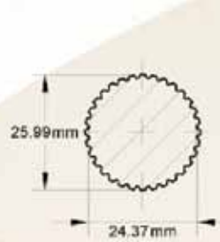
32 spline shaft cross section is 542mm sq.
