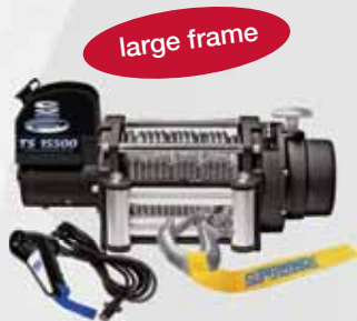
1515200 Tiger Shark 15500 Line Pull: 15,500lbs /12v Motor: Sealed 5.7 hp Wire rope: 29/64" x 94'
