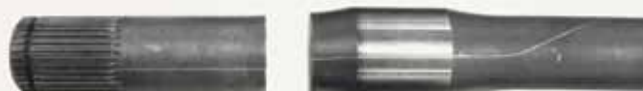
Land Rover OE front half shaft broke at 230 degrees of twist compared to the KAM shaft which twisted 540 degrees.
